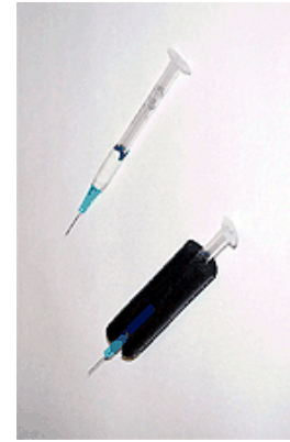
Dissecting Needle grip enlarged with foam tubing
