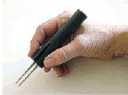
Forceps grip enlarged with foam tubing.
